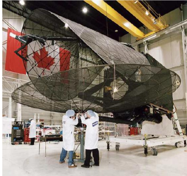
Figure 1.1 Spring back reflectors one folded (top) and one deployed (bottom), on MSAT-2 spacecraft (Courtesy of Canadian Space Agency)
