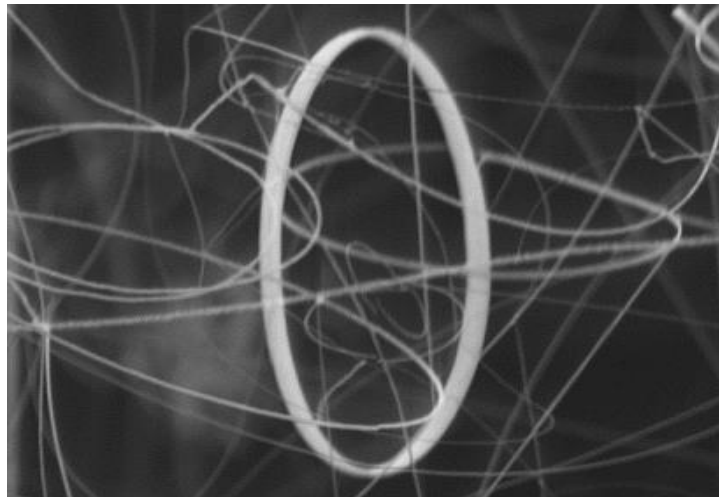
Figure 1.7. Seamless single-crystal nanorings of ZnO (Adapted from Kong et al. , 2004).
