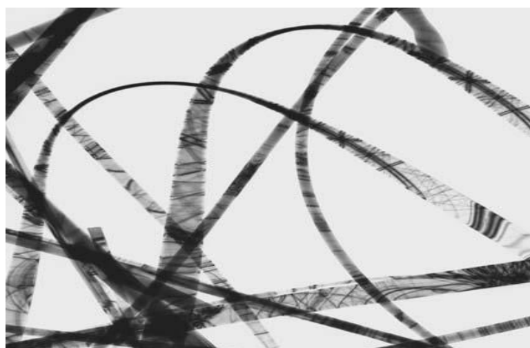
Figure 1.5. TEM image of the as-synthesized ZnO nanobelts, showing uniform morphology (Adapted from Pan et al. , 2001).
