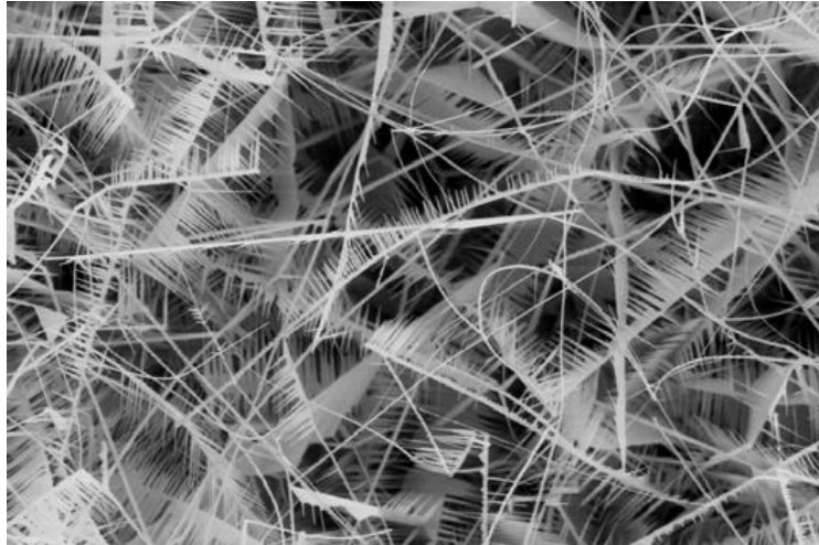
Figure 1.6. SEM image of comb-like cantilever arrays of ZnO (Adapted from Wang et al. , 2003).
