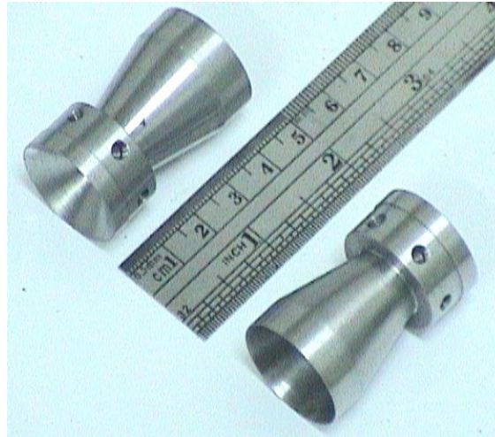
Figure 6 Convergent-divergent nozzle for rocket motor
