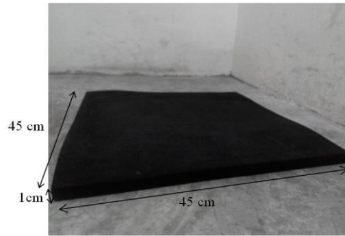
Figure 4. Fabricated single layer RHA/CNTs microwave absorber
