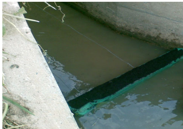
Fig. 3 The GACBF installed at mouth of the WIC
