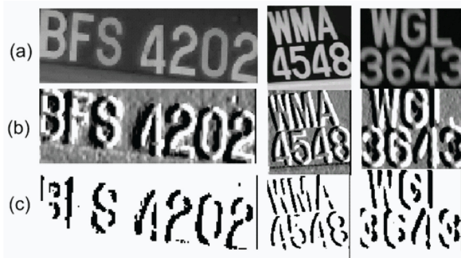
Figure 8. Examples of (a) images of detected license plates (b) image results after applying only RGB Convolution process (c) Image after applying RGB Convolution and TV1 process correspondingly
