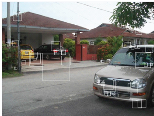
Figure 3. Samples image result using SURF technique for Malaysia license plates: Example 2
