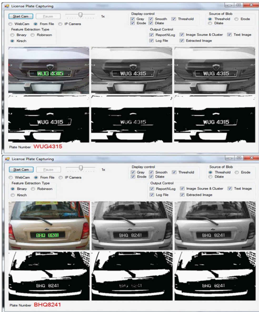
Figure 12. Examples of the correct LPD using CRLSA module
