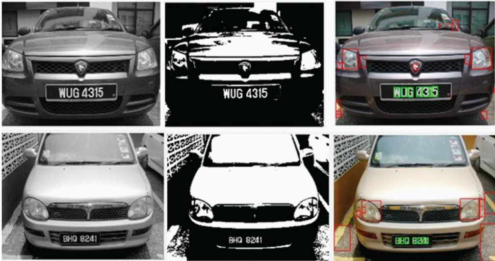
Figure 7. Examples of (left) the original, (middle) and threshold, images. While (right) are the labeled and clustered blobs images using color blob labellings process.
