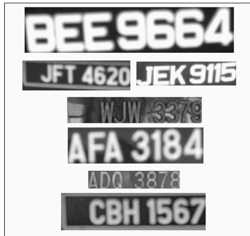
Figure 14. Fusion Images that has been successfully detected by LPD system
