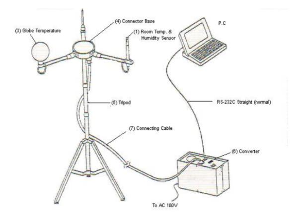
Figure 1.3 : Connection of the Comfy Meter components
