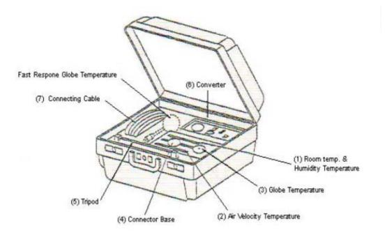
Figure 1.2 : Compartment of Comfy Meter
