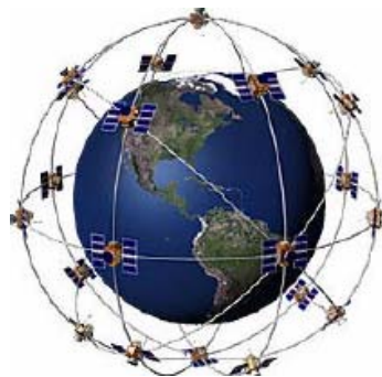
Fig. 1. GNSS Satellites Nominal Constellation
