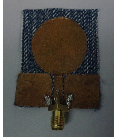
Figure 2: Fabricated antenna using denim textile
