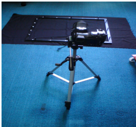
Fig. 1. Control frame used in camera calibration
