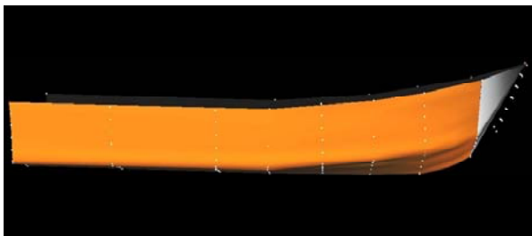
Fig. 8. The generated hull surface of model MTL 060 by photogrammetry software
