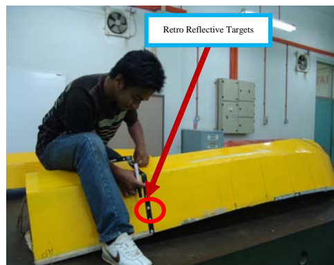
Fig. 3. Placement of retro reflective targets on model hull
