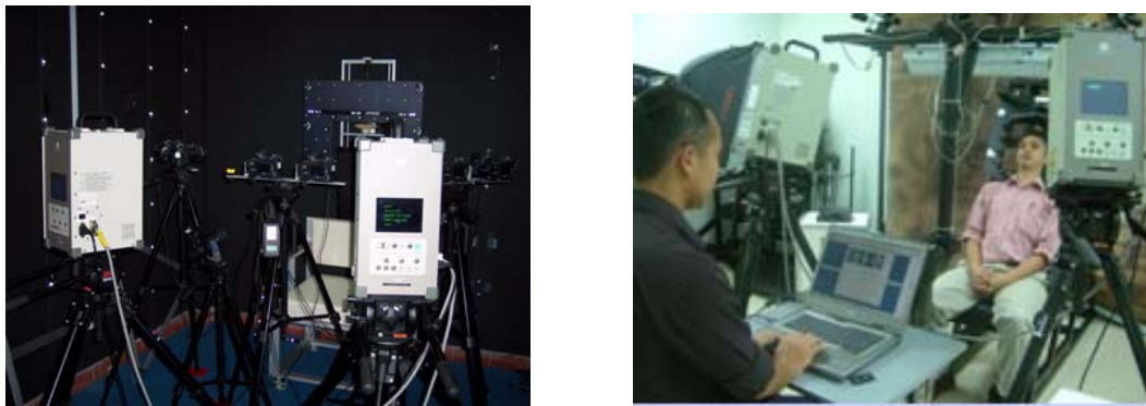
Figure 3. Real time imaging system (laser, camera, control frame)
