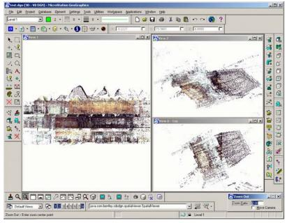
Fig. 11. 3D visualisation of point clouds, managed as points in DBMS
