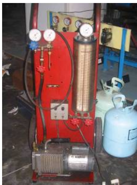
Figure H.2 Charging Equipment
