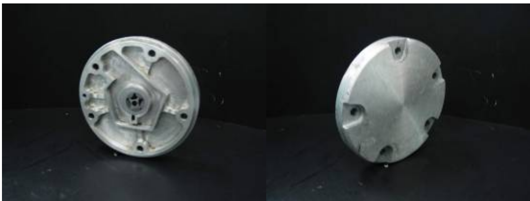
(a) (b) Figure G.3 Rear End Plate a) Front View b) Rear View
