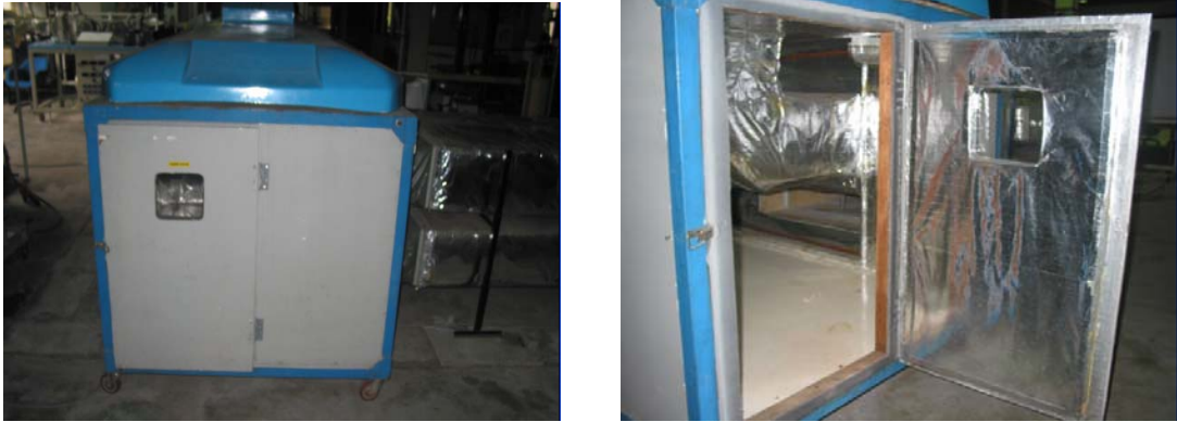
Figure 4.13 The exterior and interior views of the simulated passenger cabin
