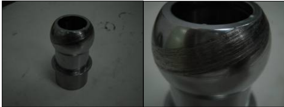
Figure L.1 Scrubbing on Ball Mount Surfaces
