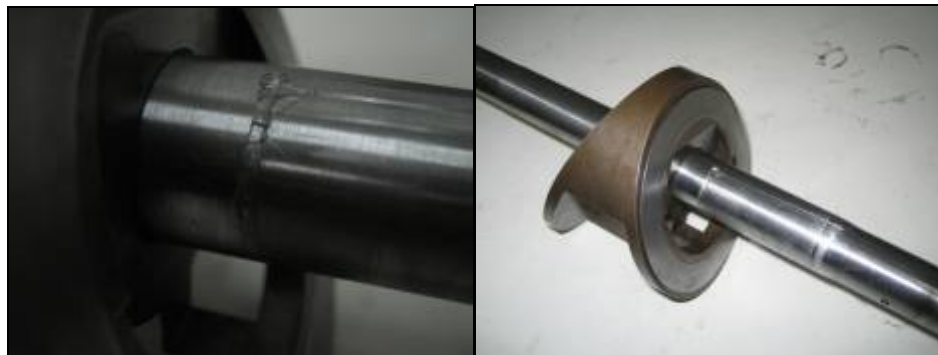
Figure L.2 Scrubbing on Shaft Surface
