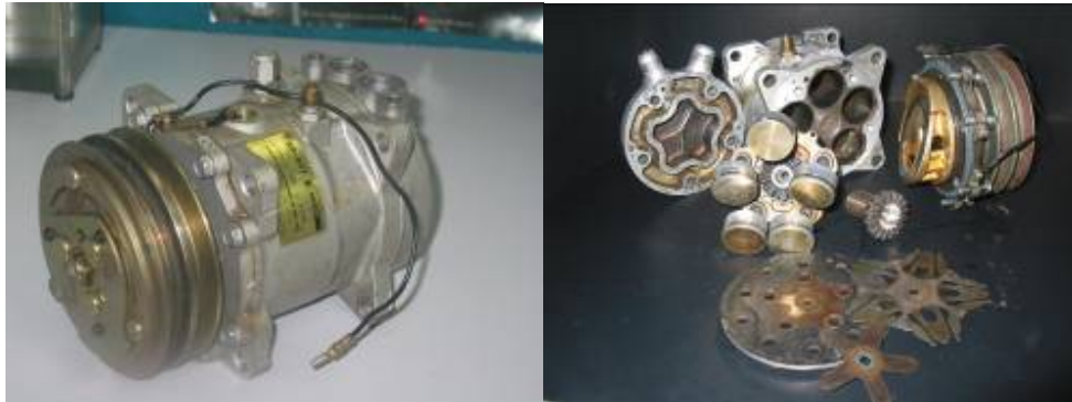
(a) (b) Figure A.1 Sanden Wobble Plate Compressor a) Compressor b) Components
