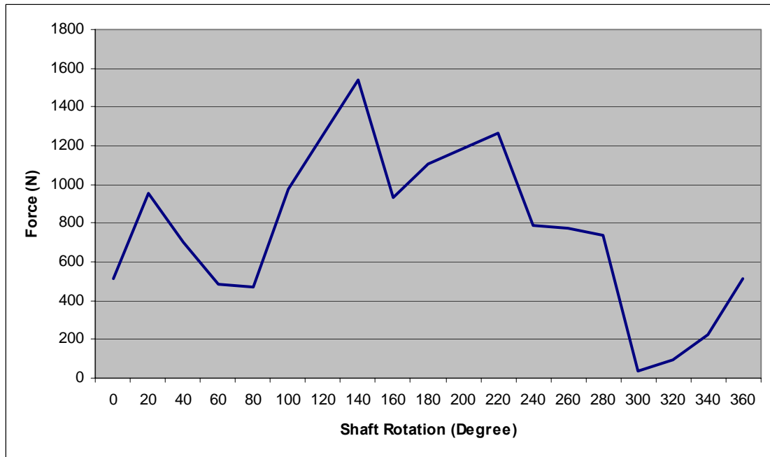
Figure 3.17 Variation of Ball Mount Reaction Force ( F_{wb} ) with Shaft Rotation Angle
