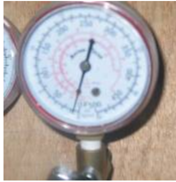
Figure I.5 (a): Pressure Gauge
