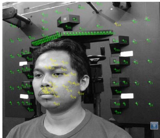
Figure 3.19: Measurement of natural features using convergent photogrammetric method
