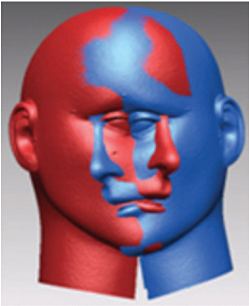
FIG. 15. Errors in the registration of the left and right scans of the 120° convergence angle.
