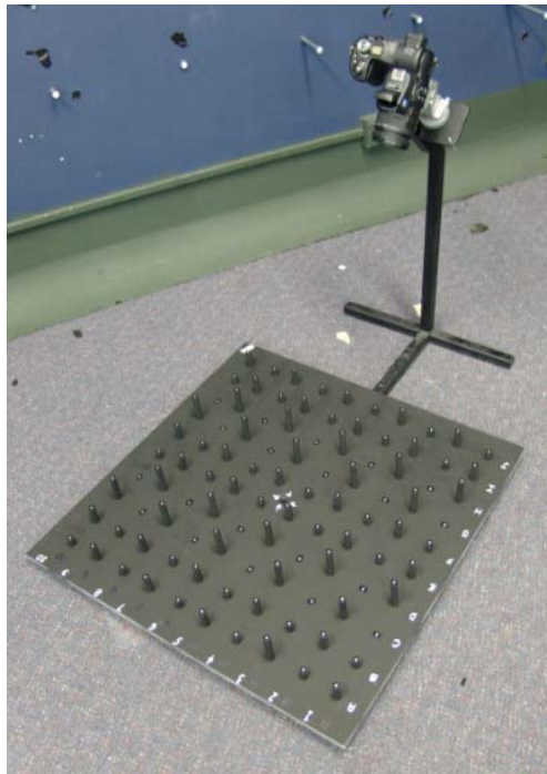
Figure 4.1: The camera calibration device
