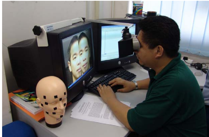
Figure 3.21: Post processing of stereo images using DVP system. Note: the 3D coordinate of the landmarks is measured in 3D environment through stereo imaging devices.
