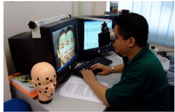
Figure 4 Stereo digitizing using Digital Video Plotter (DVP) Photogrammetric Workstation.
