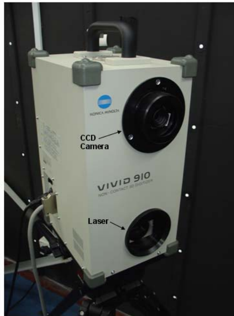
Figure 3.9: The Minolta VI-910 3D laser scanning system
