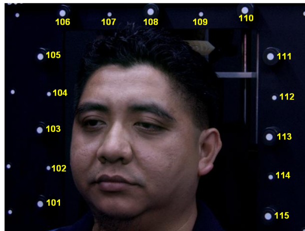
Figure 5.9: Location of photogrammetric targets used in the study
