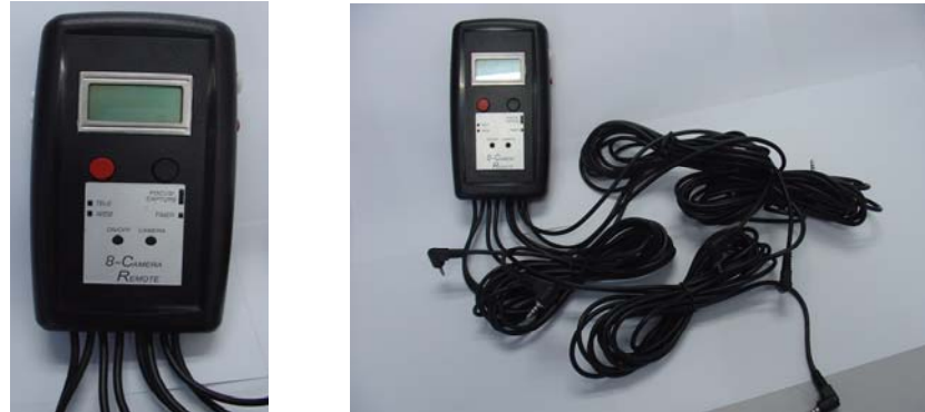
Figure 3.5: The camera controller and synchronization device
