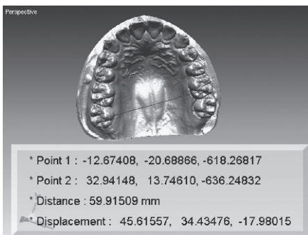
Figure 7: Slope distance measurement on dental cast surface 3D model.
