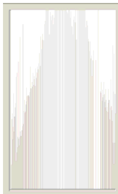
Figure 3.17 The histogram after histogram equalization
