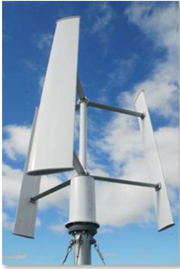
Figure 1.1 Straight-Bladed VAWT (Travis Justin Carrigan, 2010)
