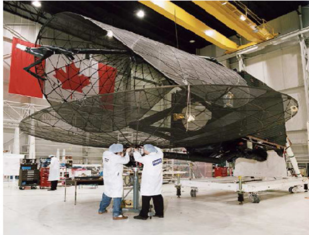
Figure 1.2: Spring back reflectors of MSAT-2 spacecraft (Courtesy of Canadian Space Agency)
