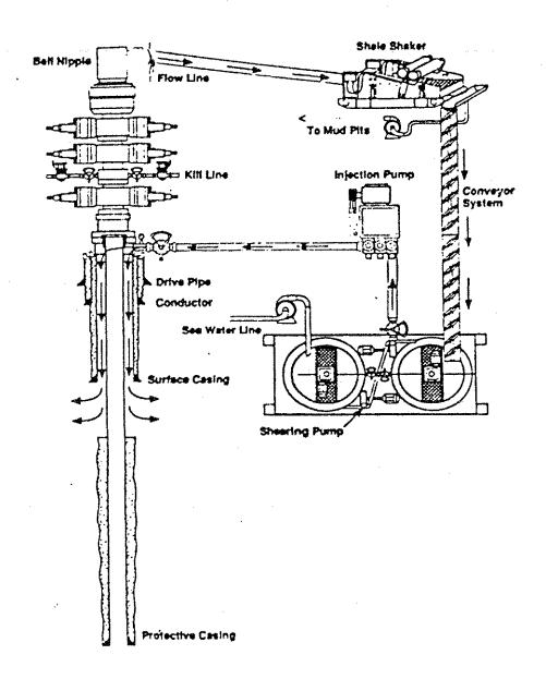
Figure 1: OBM Cuttings Shearer Process Schematic (Sirevag and Bale, 1993)
