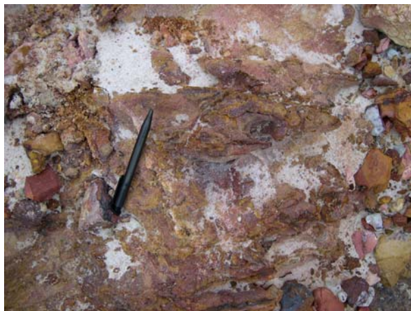
Figure 7.4: Presence of thick iron pan (4 cm) on grade IVa sandstone resisting the penetration of ripper tine
