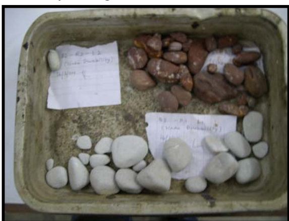
Figure 4.18: Samples after being tested by the slake durability Testing
