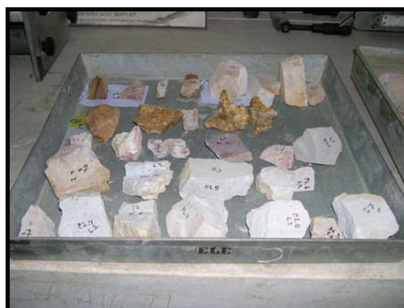
Figure 4.17: Samples prepared for slake durability testing
