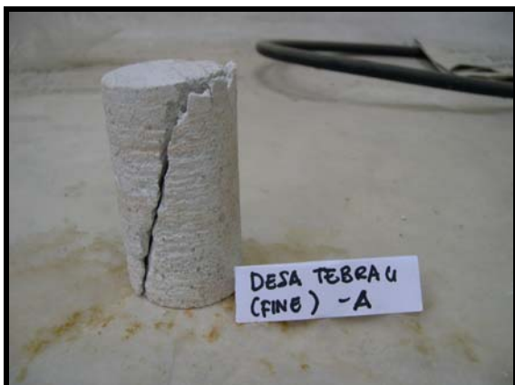
Figure 4.14: Sample tested by UCS
