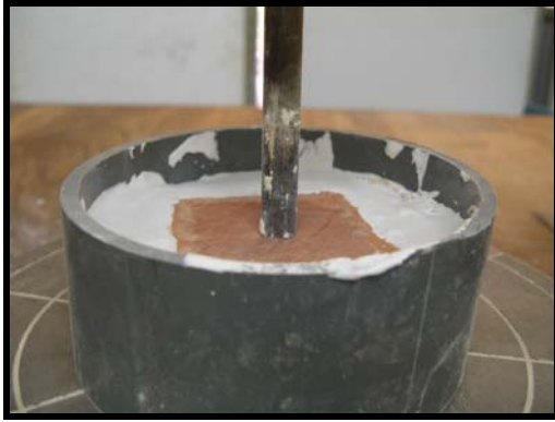
Figure 4.19: Penetration test by using a 10mm bit probe
