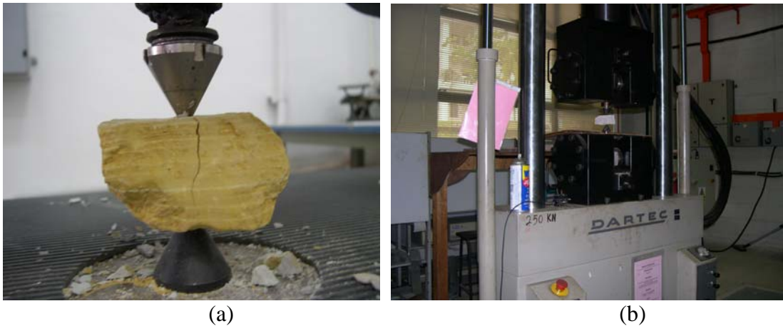
Figure 6.6: Photographs showing samples tested by the point load test (by UTM): (a)- (sample R2L1), (b)- sample B8L9 tested by UTM
