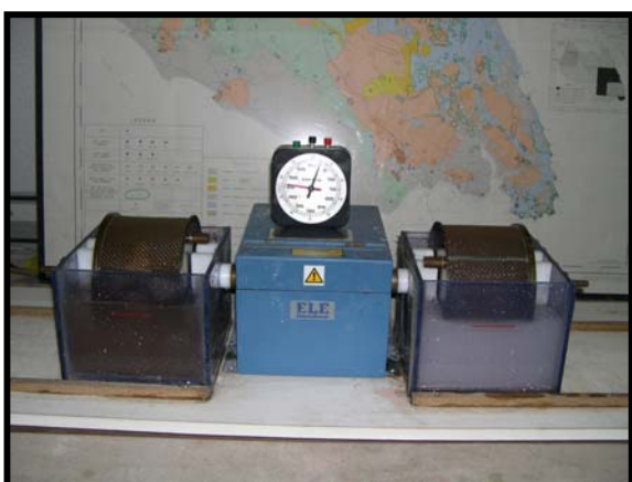
Figure 4.16: Apparatus for slake durability testing
