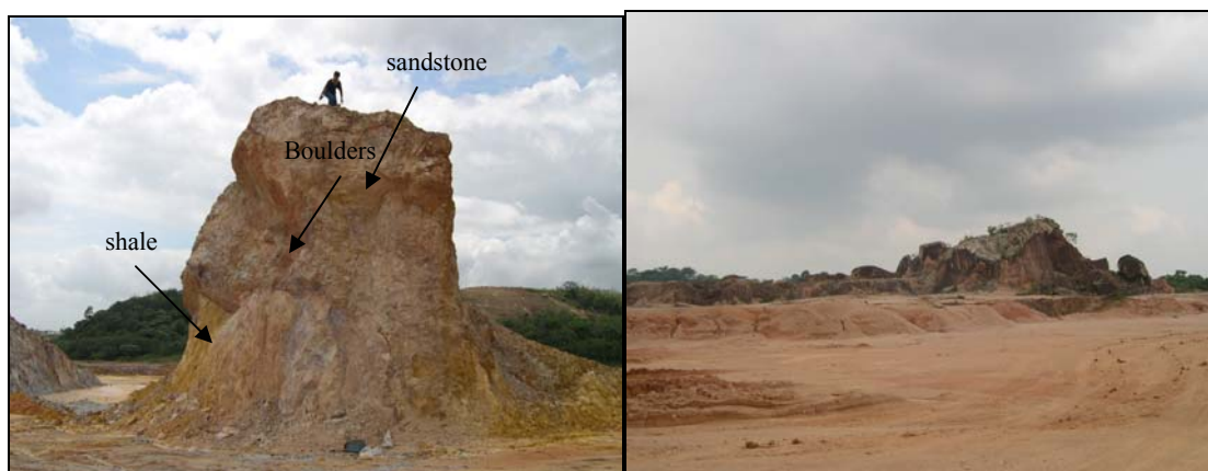
Figure 2.2: Interbedding of sandstone grade II (top layer) and shale grade V (lower layer) (Location: Bukit Indah)
