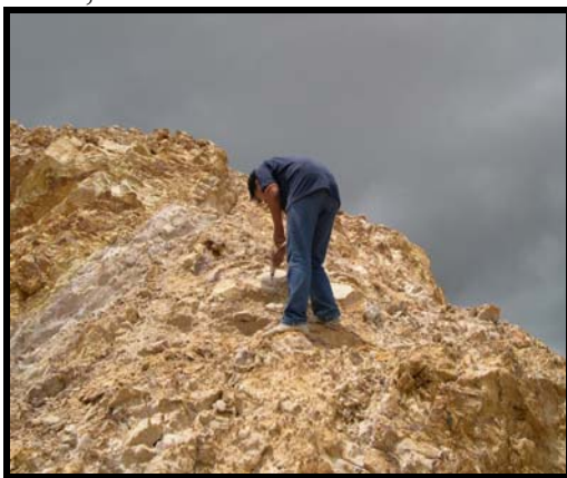
Figure 4.6: Performing Schmidt Hammer Test at Layer 2 (sandstone grade IVa), B7 Bukit Indah, Johor
