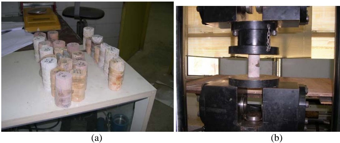
Figure 6.7: Photographs showing samples tested for UCS: (a)- some samples being tested by UCS, (b)- samples tested by the Universal Testing Machine (UTM)
