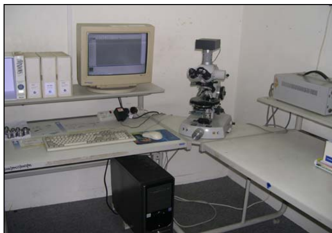
Figure 4.21: A Carl Zeiss Axiocam with KS300 image analyzer system that being used for petrographic analysis
