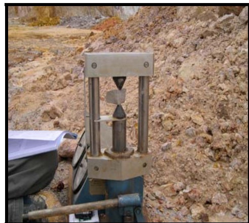
Figure 4.7: Testing on Portable Point Load at the site
