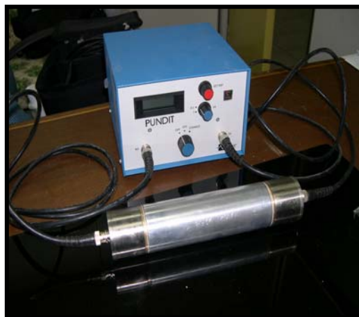
Figure 4.8: PUNDIT Test Equipment
