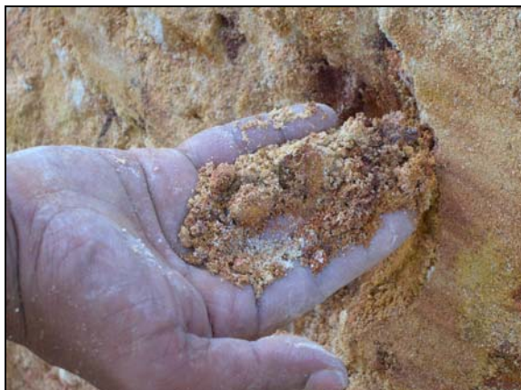
Figure 2.1: Grade IV sandstone can be very friable when moisture content is high
