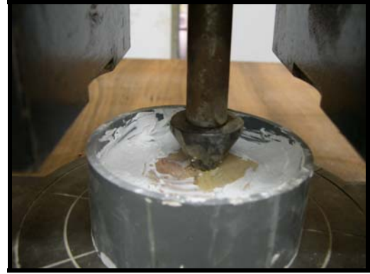
Figure 4.20: Penetration by using a point load bit
