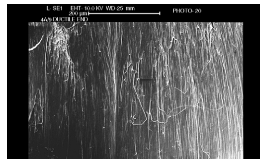
Fig. 4. SEM micrograph of blend M1 sample showing ductile failure.
