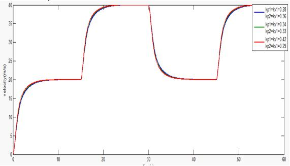
Figure 5. Speed response with fixed time headway for various kp and kvvalues and vehicle dynamics
