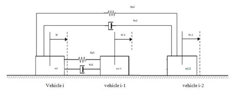
Figure 2. A mathematical model of a vehicle convoy system control strategy.
