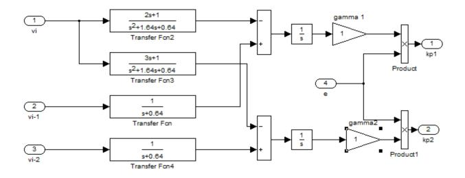
Figure 9. Simulation diagram of adaptive mechanism
