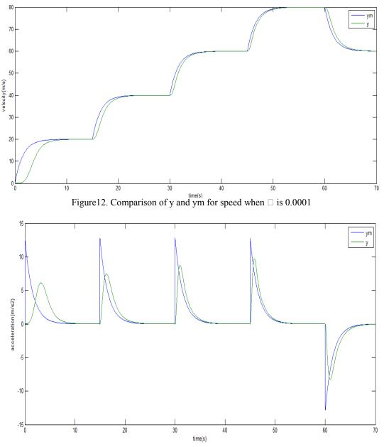
Figure 13. Comparison of y and ym for acceleration when  $\Box$  is 0.0001
