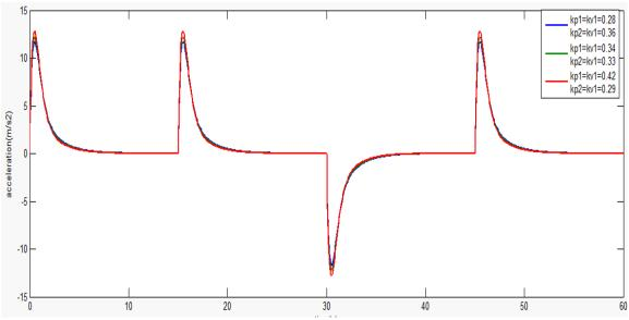
Figure 6. Acceleration response with fixed time headway for various kp and kvvalues and vehicle dynamics
