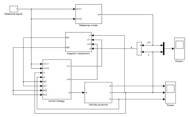
Figure 8. The gradient approach adaptive gain controller simulation diagram
