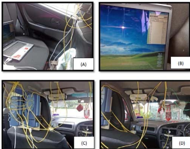
Figure 11 Experiment apparatus: (A) USB TC-08 is connected to a laptop; (B) Temperature reading displayed on line; (C) USB TC-08; (D) Thermocouples arrangement.
