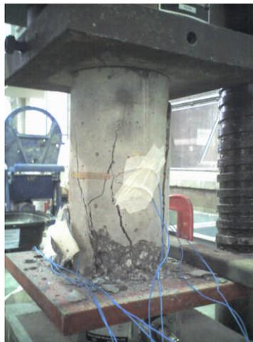
Figure 11. Static modulus of elasticity test
