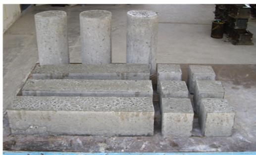
Figure 2. Hardened concrete after opening the mould for 24 hours
