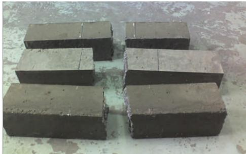
Figure 8. The prism failed after flexural testing
