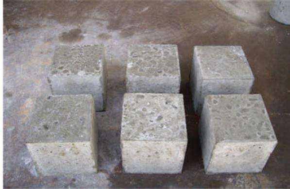
Figure 3. Hardened cube concrete for 7 and 28 days curing
