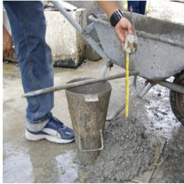
Figure 1. The process of Slump test measurement
