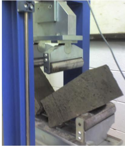
Figure 7. The process of flexural Strength Test
