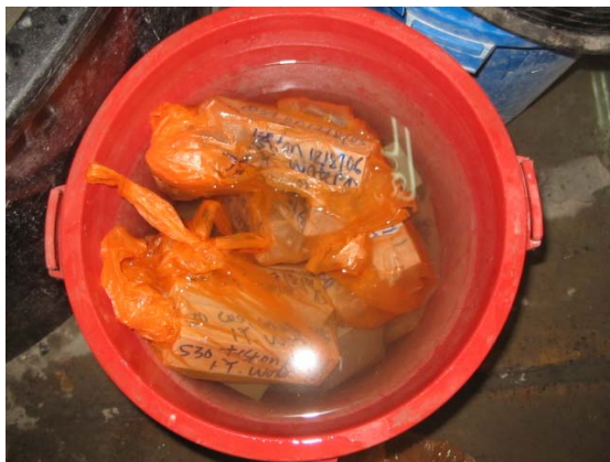
Fig. 3: Continuous water curing at 25 – 26 o C
