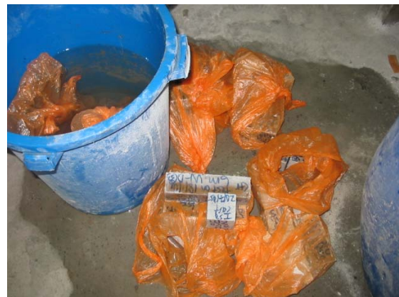
Fig. 4: Wet-dry cycles. Immersed in water per week and exposed to open air per week consider as one cycle
