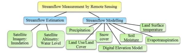
Figure 1. Role of remote sensing in streamflow measurement.
