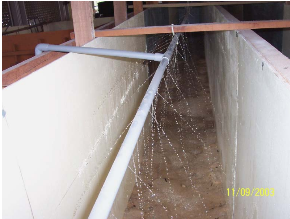
Figure 3.5: Rainfall Pumping into the Laboratory Model for Infiltration Test
