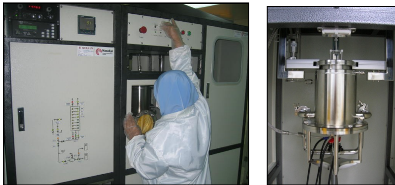
Figure 7: The author with the MOCVD system at IIS, UTM. Picture on the right side is the vertical chamber which the sources gas mixed to produce epitaxial layer (in front of the author).
