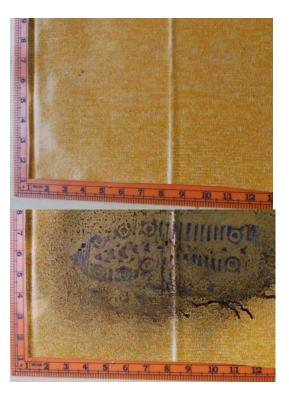
Fig. 5: The mud stained shoeprint mark on linoleum before (Top) and after (Bottom) treatment with sudan black
