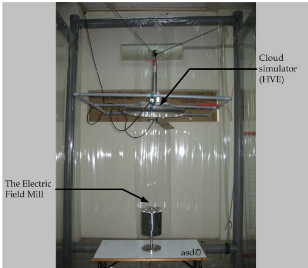
Figure 3.12 The REFEM calibration setup
