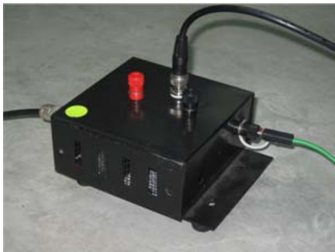
Figure 2. 3 Pictorial view of leakage current sensor box
