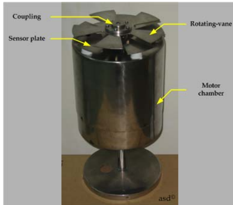
Figure 3.2 Rotating-vane type EFM
