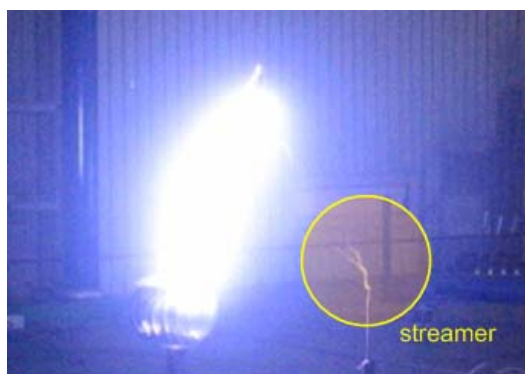
Figure 4. 17 A result of lightning impulse discharge of the competitive test for the first prototype where the upward streamer was also developed on the tips of the conventional LAT.
