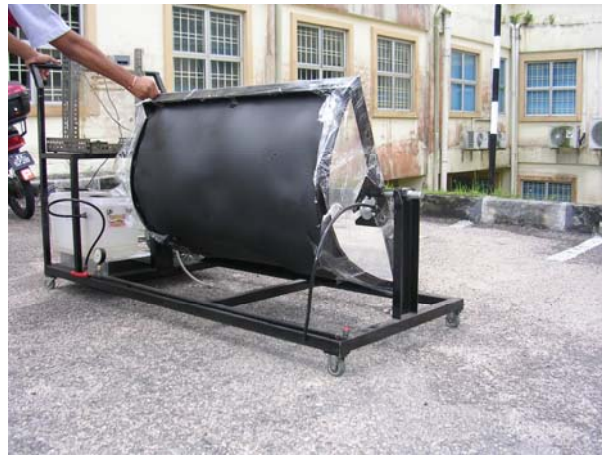
Figure 5.29: View of Solar Test Rig Wrapped and Insulated
