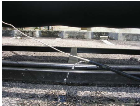
Figure 5.32: Absorber Outlet Temperature ( T_{out} ) Taken Using a Thermocouple
