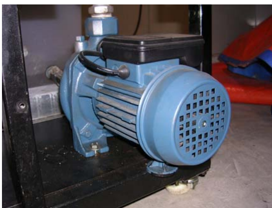
Figure 5.20: Pump capacity 0.5hp
