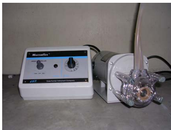
Figure 5.21: Pump capacity 0.1hp
