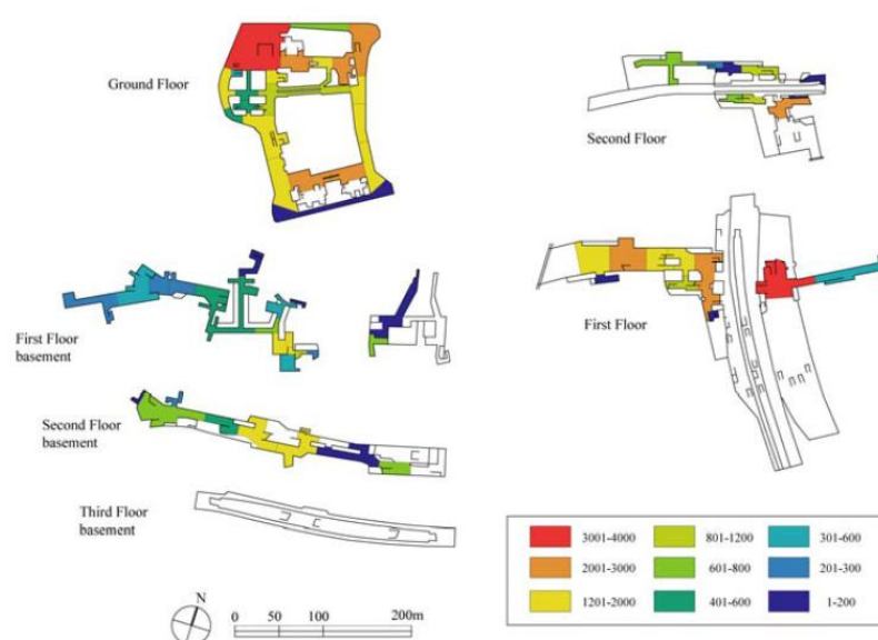
Figure 1-3 The number of pedestrians flow in block per ten minutes in the case of Shibuya Station, Tokyo, Japan
