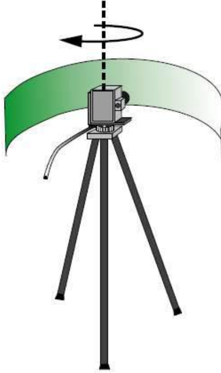
Figure 3: Turning the camera on the tripod about the optical centre of the camera clockwise direction
