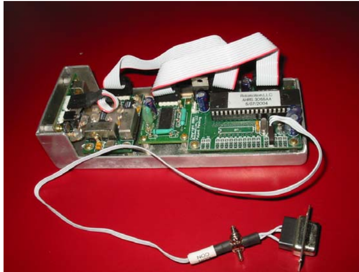
Figure 5 The low dynamic AHRS (AHRS3050AA) from Rotomotion, LLC. This AHRS operated at slower updated rated (30Hz) and output the attitude measurement via serial port compare to other high end AHRS from Rotomotion, LLC.
