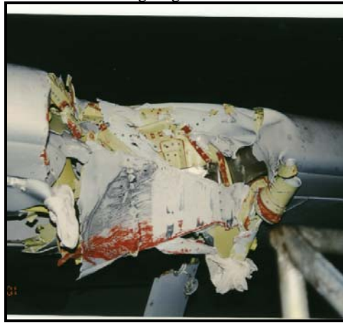
Figure 5: Exploded View of Damaged Wing Leading Edge Structures
