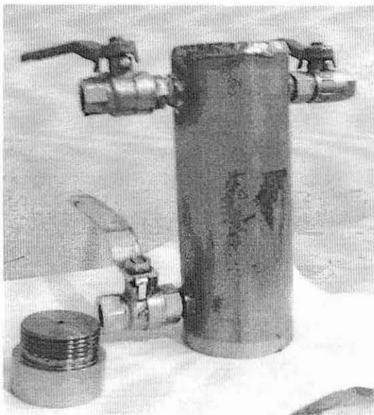
Fig. 2 An example of the actual stainless steel test tube used for the ageing tests
