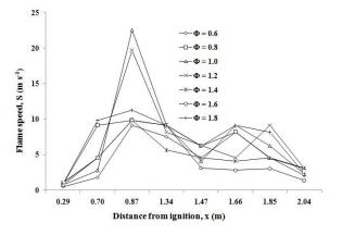
Figure 5 Flame speed profile against distance from ignition at various mixture concentrations on straight pipe
