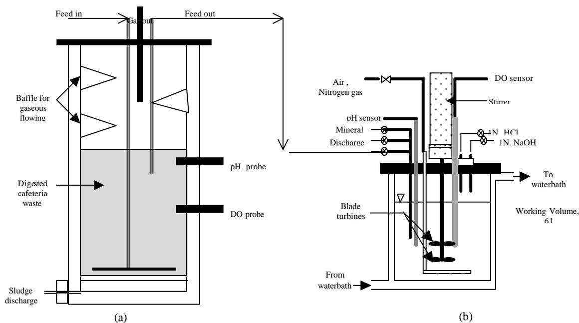
Fig. 1—Experimental set-up of combined (a) UASB and (b) Bio-PORec® reactor
