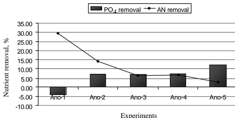
Fig. 2—Nutrient removal at different anoxic/aerobic conditions
