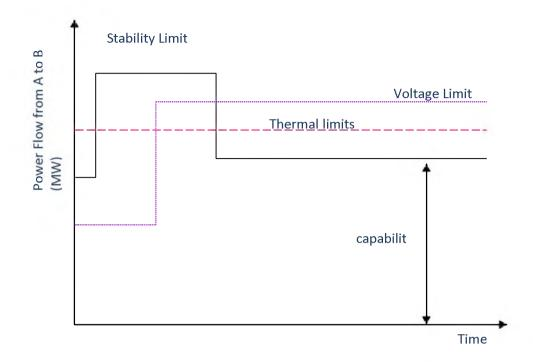
Figure1 Total transfer capability changes in different time frames.
