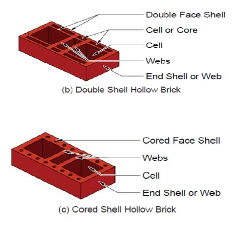
Figure.1.1 Hollow brick configuration
