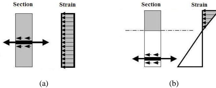
Figure 1.1: (a) Stress transfer in pull-out test, (b) Stress transfer in beam test
