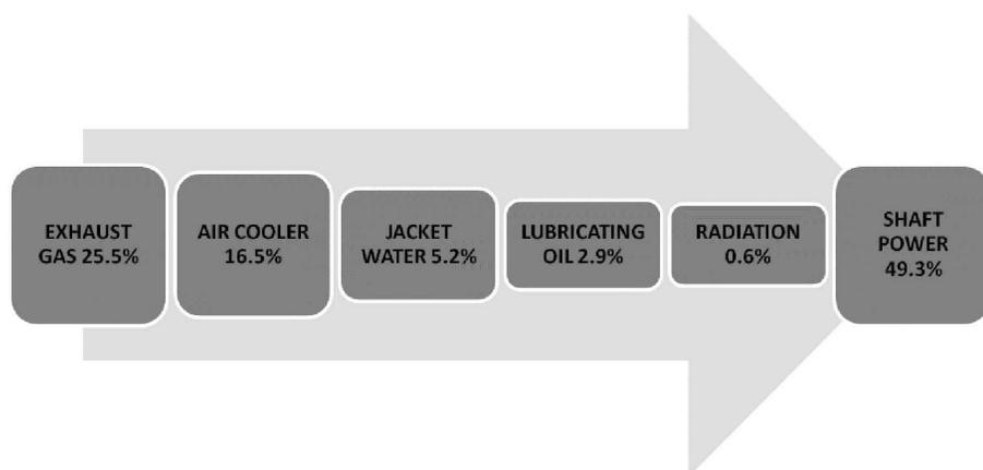
Fig 1: Heat balance of a modern large diesel engine
