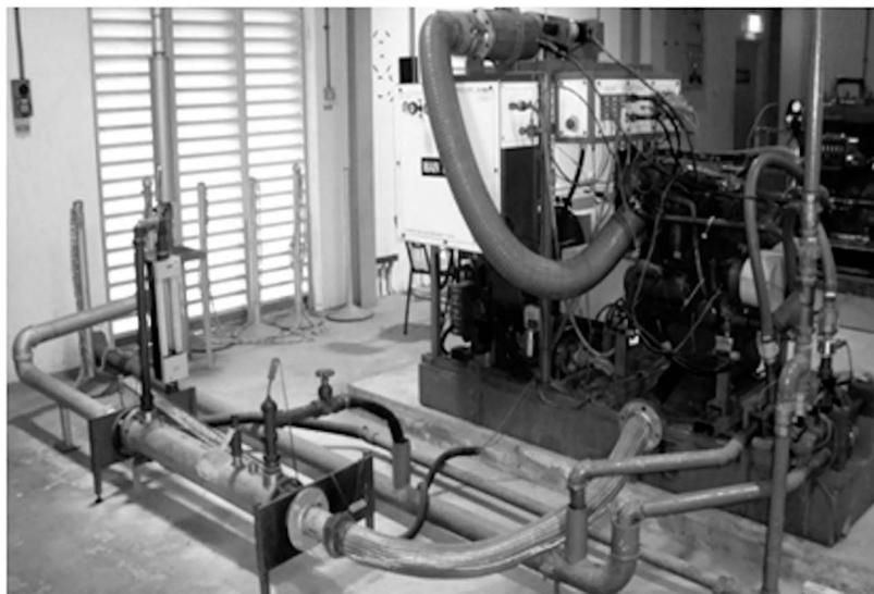
Fig 3: Testbed engine with exhaust gas calorifier arrangement
