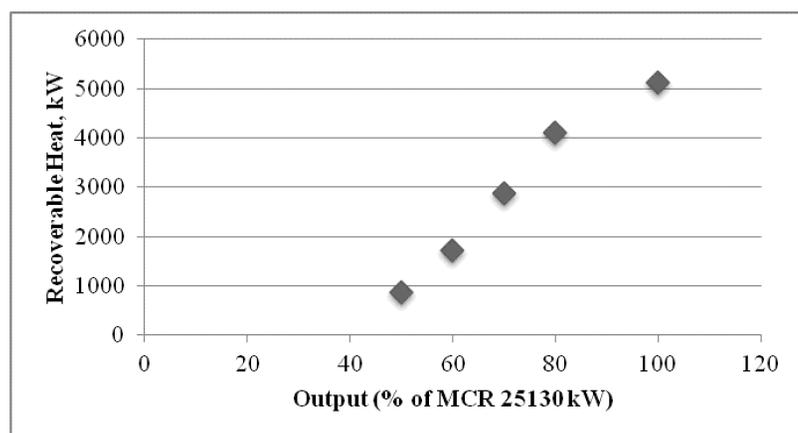
Fig 4: Possible heat recoveries from ME after turbocharger and EGE
