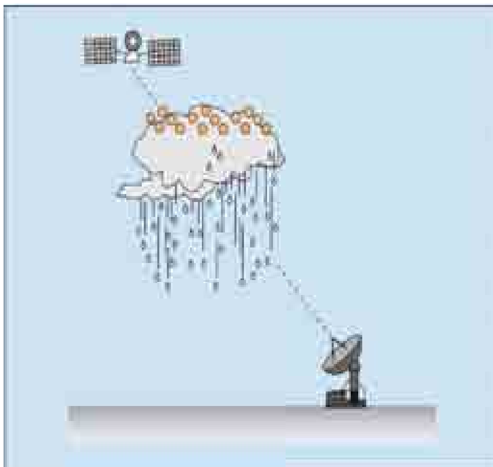
Figure 1.1: Effect of Rain on the Satellite Link
