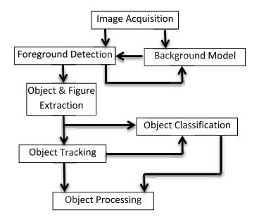
Figure 1: Automatic aerial video surveillance system.
