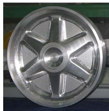
Fig. 12. The product after cutting process
