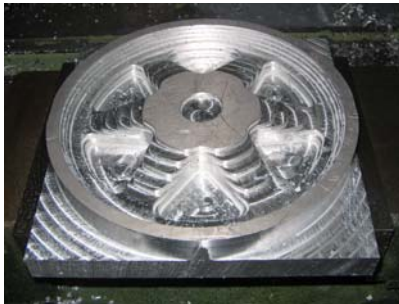
Fig. 9. After roughing process
