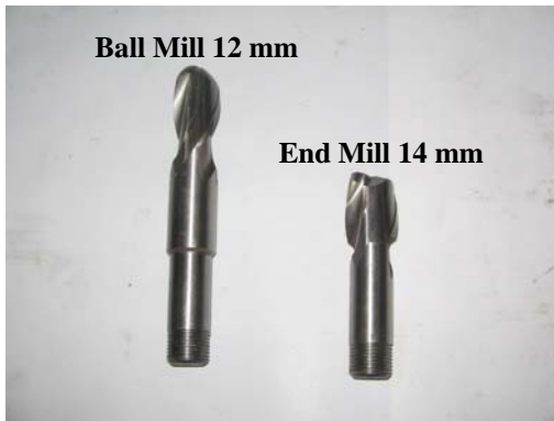
Fig. 8. Machine tools for real machining process
