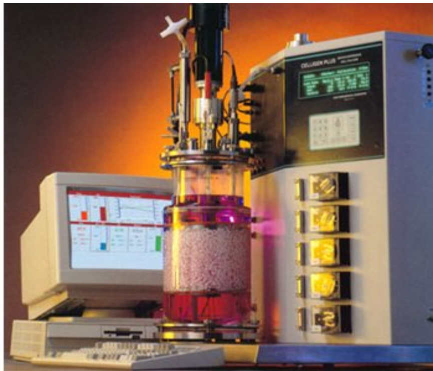
Eg: CelliGen Plus, an all-purpose stirred-tank bioreactor
