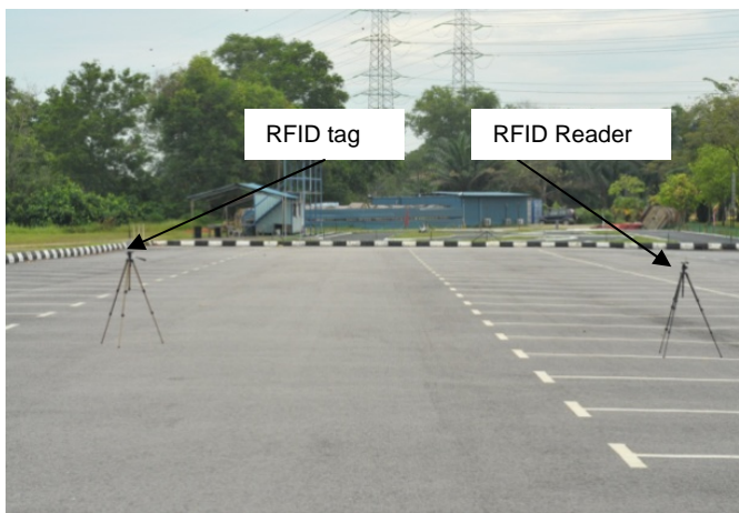
Figure 7 Measurement setup at Padang Kawad (Open Space)
