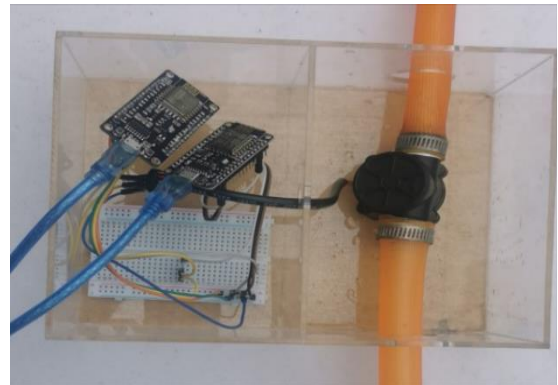
Fig. 14. Smart Water Meter based IoT.
