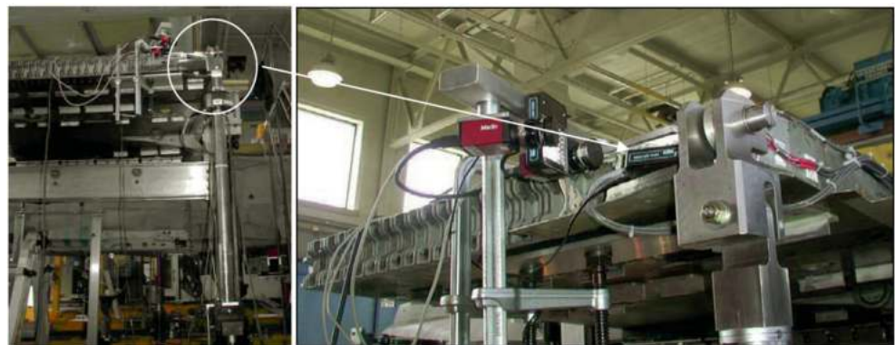
Figure 2. Fatigue test setup rig [26].
