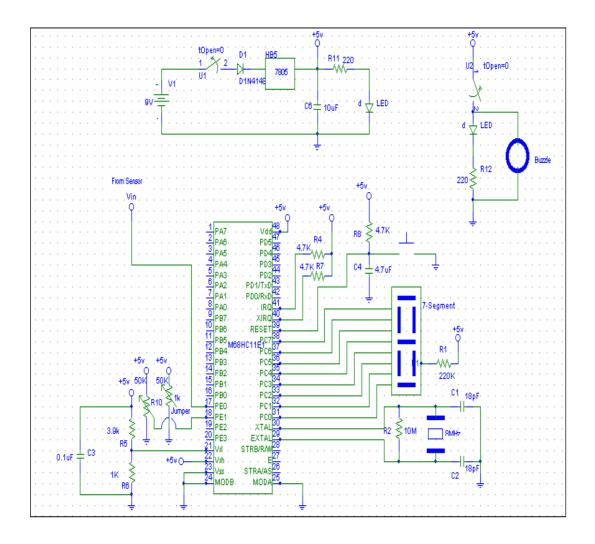
**Figure 6.7 Controller Module Circuits**
