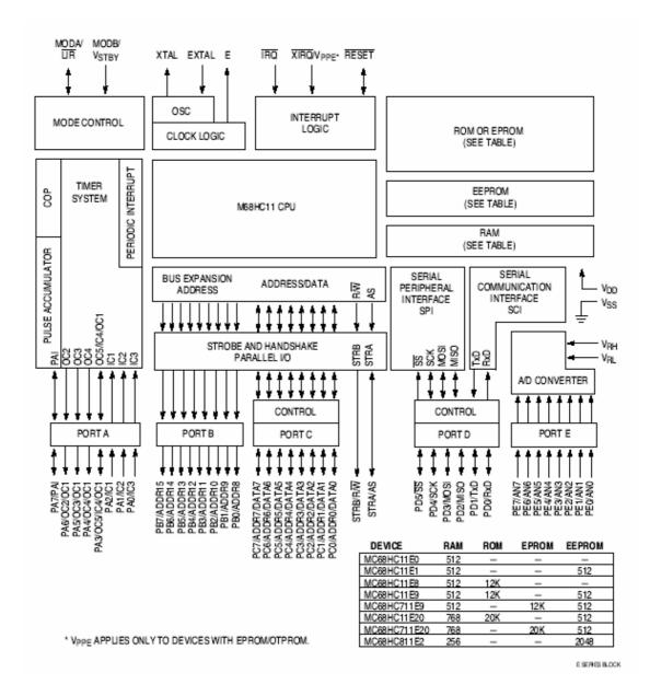
Figure 3.1 M68HC11 E-series block diagram
