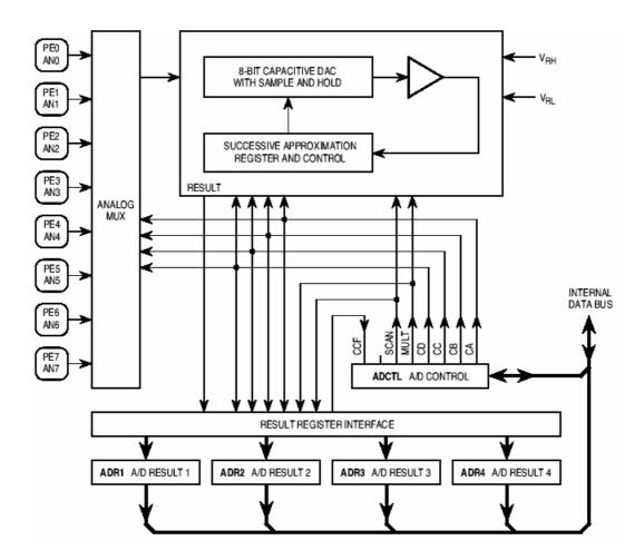
Figure 3.7 A/D Converter Block Diagram
