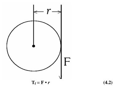
Figure 4.8 Frictional torque is the force (F) required to move a load multiplied by the length of the lever arm (r)
