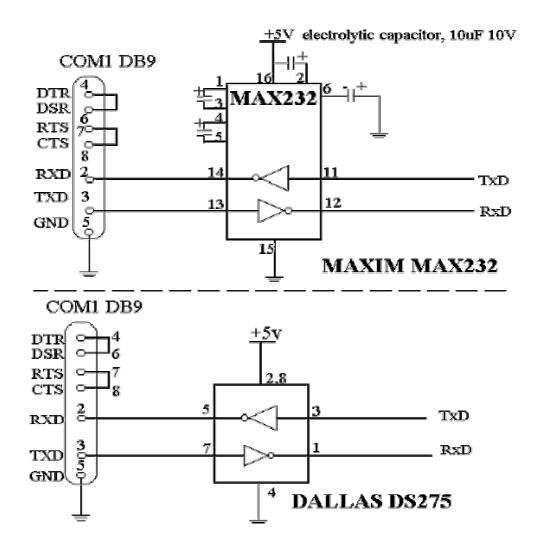
Figure 6.9 The connection of MAX 232C and DS275 for communication between PC and Microcontoller chip.
