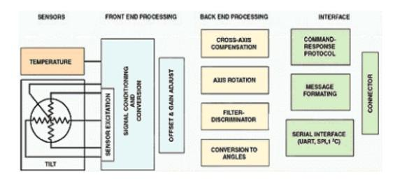
Figure 2.3 Hardware and firmware functions are performed by a high-end, microprocessor-based, dual-axis inclinometer.
