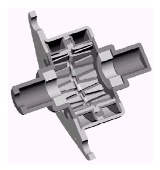
Figure 4.7 Partial cut away showing pole plates of a  $7.5^\circ$  step angle motor
