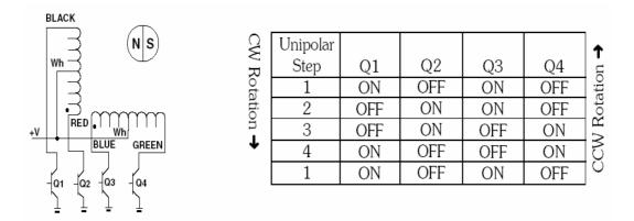
Figure 4.6 Wiring diagram and step sequence for unipolar motor.
