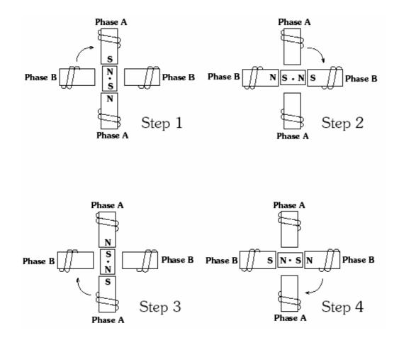
Figure 4.2. "One phase on" stepping sequence for two phase motor
