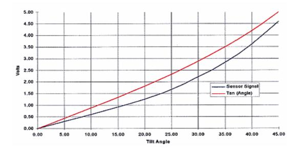
Figure 2.4 Tilt sensor signal plotted against the ideal tangent response, note that above 20° the signal output becomes nonlinear and requires calibration.
