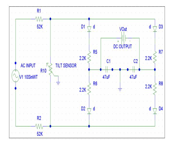
Figure 6.4 AC To DC Conversion Circuits
