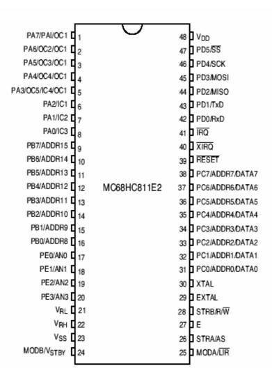
Figure 3.2 Pin Assignments for 48-Pin DIP (M68HC811E2)
