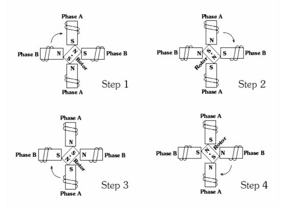
Figure 4.3. "Two phase on" stepping sequence for two phases motor
