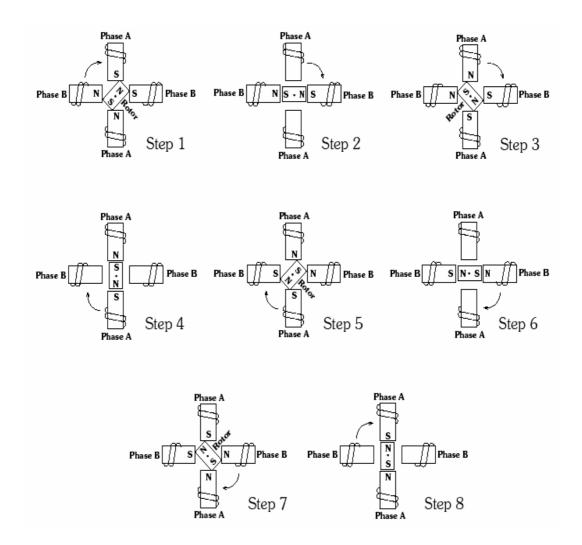
Figure 4.4 Half-stepping –  $90^{\circ}$  step angle is reduced to  $45^{\circ}$  with half-stepping.
