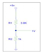
Figure 6.5 Voltage Divider Circuits Give 5V and 1V
