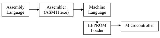
Figure 3.4 The Flow of Programming M68HC11 E Series
