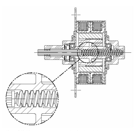
Figure 4.10. Linear actuator cut away showing threaded rotor to lead screw interface.
