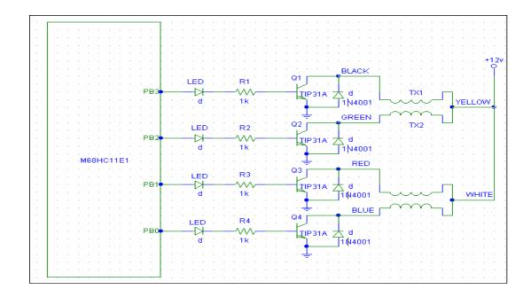
**Figure 6.12 Motor Switching Circuits**
