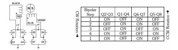
Figure 4.5 Wiring diagram and step sequence for bipolar motor.
