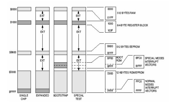
Figure 3.5 Memory Map for MC68HC11E0, MC68HC11E1, MC68HC11E8, and MC68HC(7)11E9
