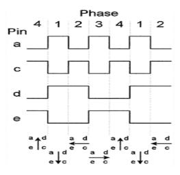
Figure 2.2 The arrows indicate the direction of current flow that occurs when voltage waveforms apply simultaneous excitation to four outer pins
