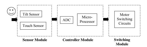
Figure 6.2 System Architecture
