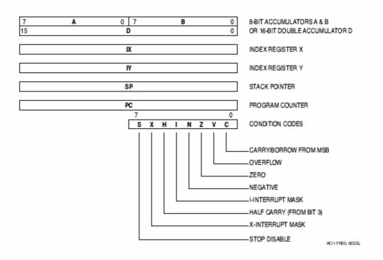
Figure 3.3 Programming Model For M68HC11 E Series
