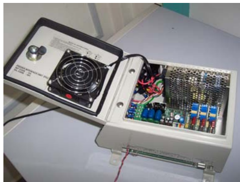
Figure 2.4: Feeder Interface Unit (FIU).
